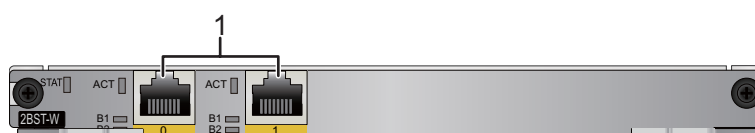
Figure 6-181 Interfaces on a 2BST-W card
