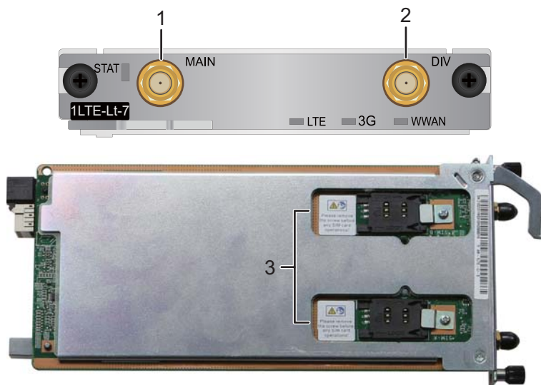
Figure 6-147 Interfaces on a 1LTE-Lt-7 card
