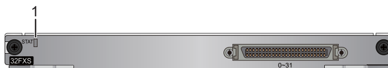
Figure 6-190 Indicators on a 32FXS card
