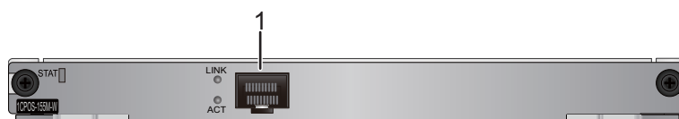
Figure 6-163 Interfaces on a 1CPOS-155M-W card
