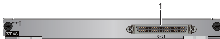
Figure 6-191 Interface on a 32FXS card
