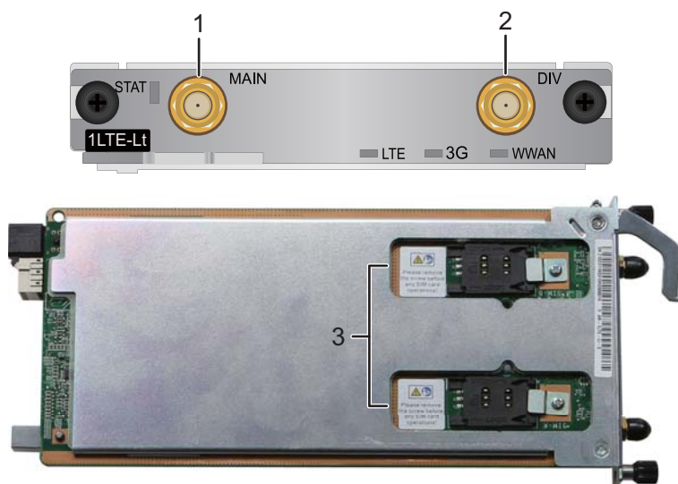
Figure 6-144 Interfaces on a 1LTE-Lt card
