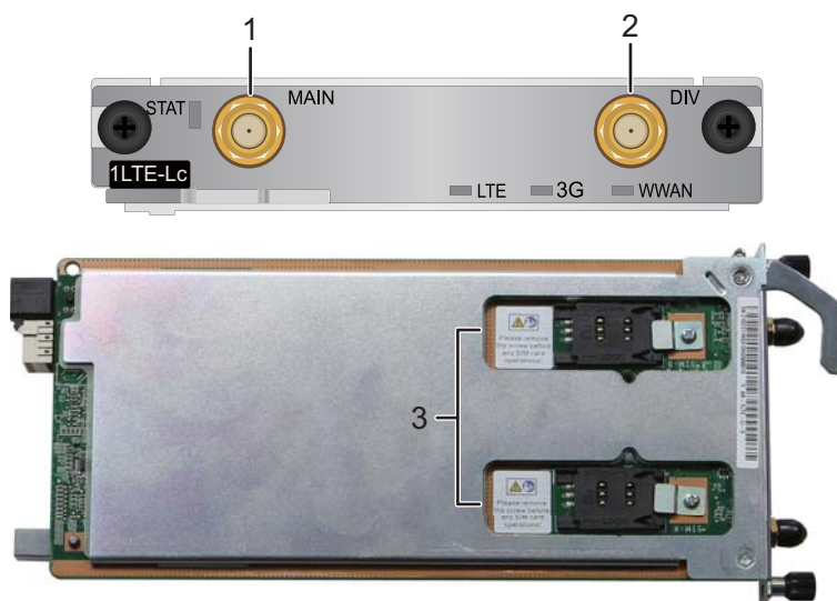
Figure 6-153 Interfaces on a 1LTE-Lc card
