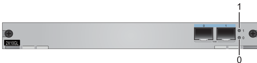
Figure 6-74 Indicators on a 2X10GL card
