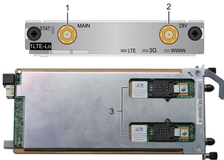
Figure 6-150 Interfaces on a 1LTE-Lo card
